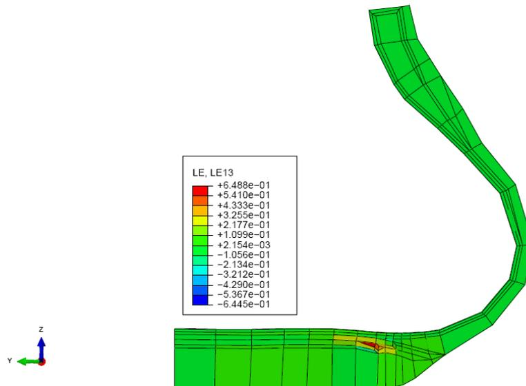
**Fig.8:** Shear strain concentrated on belt edge from 3-D FE simulation
