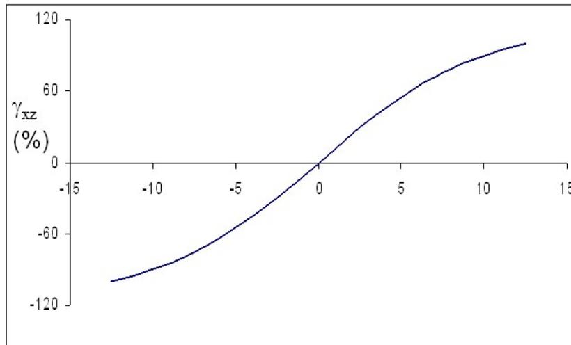
**Fig.3:** Interlaminar shear strain (xz) vs. position along belt width (when  $E_x=20\%$ , belt angle= $\pm 22$  deg.)<sup>[2]</sup>
