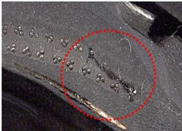
**Fig.4:** Small crack initiated from the belt edge between the two steel belt plies.
