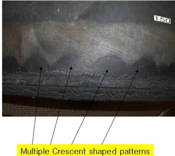
**Fig.5:** Crescent shaped patterns on a belt-leaving-belt tread separation incident.
