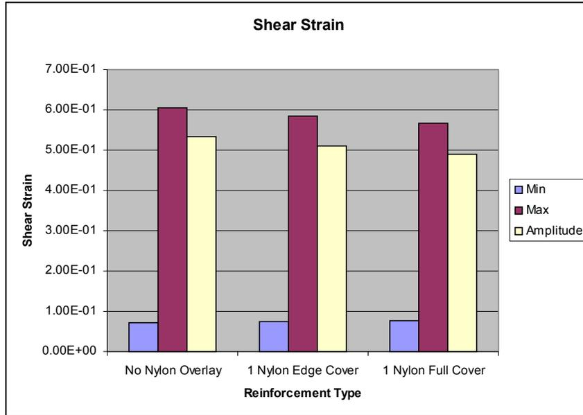
**Fig.9:** Shear strain and shear strain amplitude by reinforcement type.
