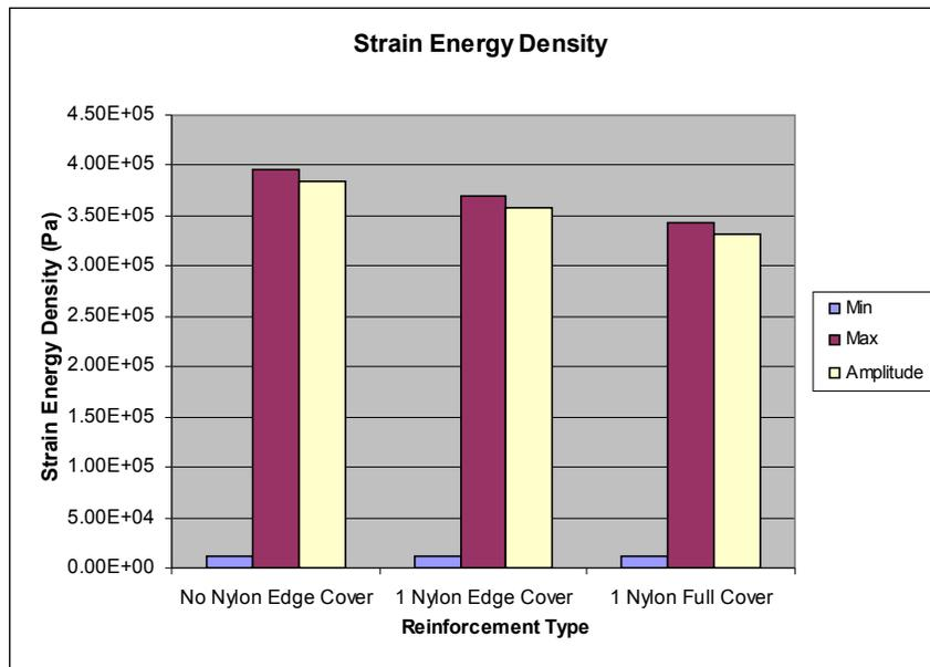
**Fig.10:** Strain energy density (SED) and SED amplitude by reinforcement type.
