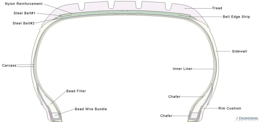
**Fig.6** 2-D Section View of a P-metric Tire
