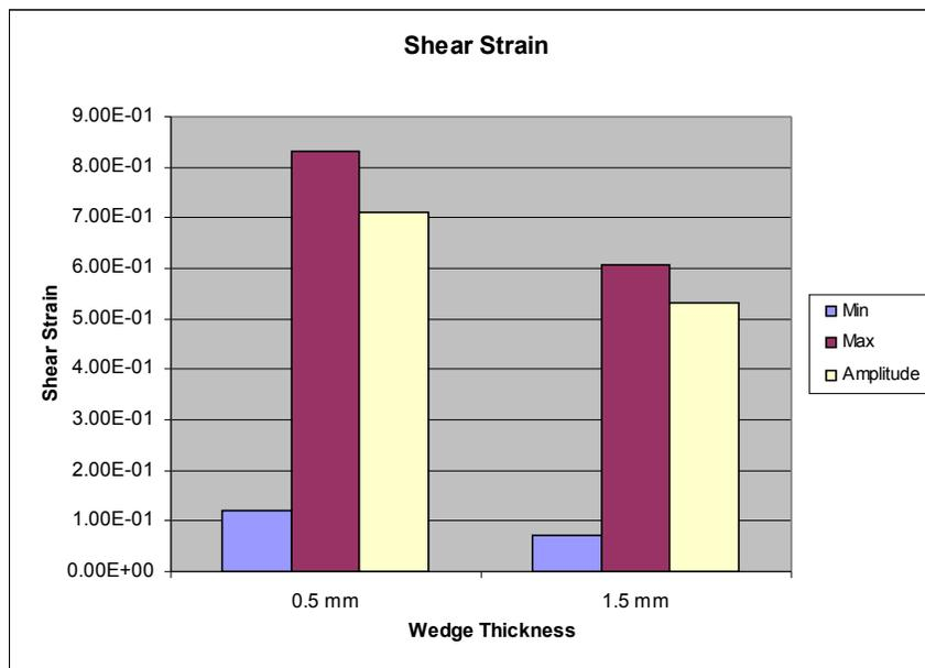
**Fig.12:** Shear strain and shear strain amplitude by belt edge strip thickness.
