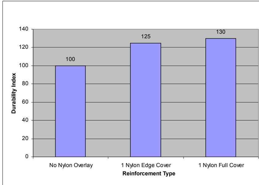
**Fig.11:** Drum test data showing nylon overlay reinforcement effect (Data courtesy of Q Tires Inc. Greenville, SC)
