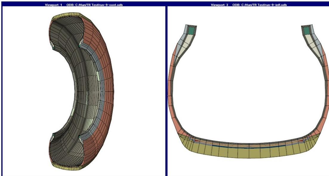
**Fig.7** Three dimensional FE model
