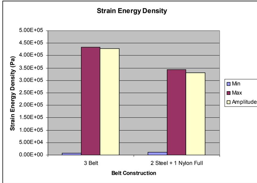
**Fig.16:** Strain energy density (SED) and SED amplitude by belt package.
