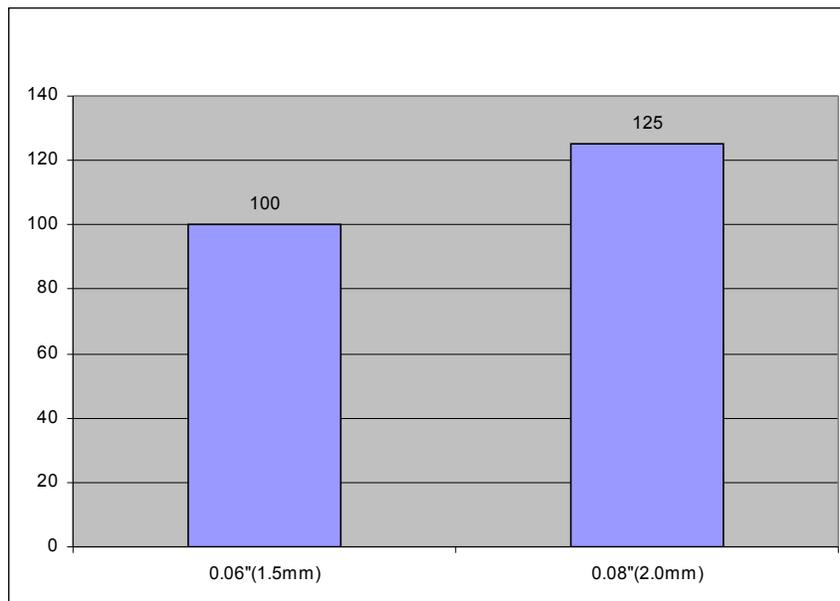
**Fig.14:** Drum test data showing belt edge strip gauge effect (Data courtesy of Q Tires Inc. Greenville, SC)
