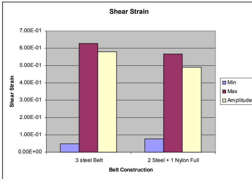
**Fig.15:** Shear strain and shear strain amplitude by belt package.
