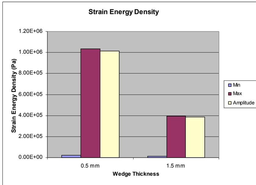
**Fig.13:** Strain energy density (SED) and SED amplitude by belt edge strip thickness.
