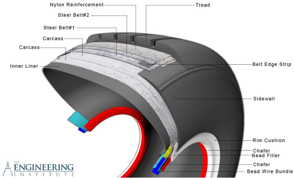
**Fig.1:** Cutaway view of a typical passenger radial tire.
