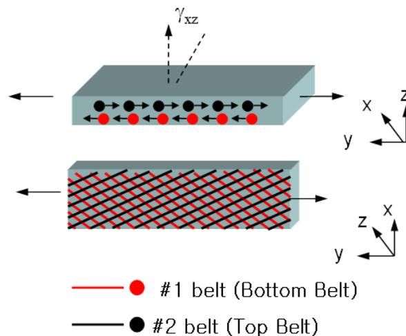
**Fig.2:** Belt layers and shear strain under extension.
